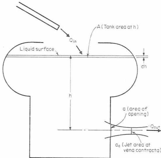
Fig. 35 Notation for tank flow
