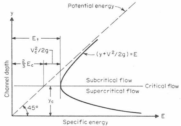
Fig. 34 Specific-energy diagram, constant flow rate.
