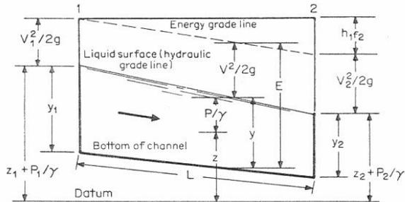
Fig. 33 Notation for open-channel flow.
