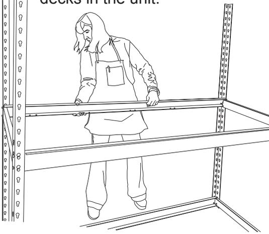
**Step 6** Screw the deck supports to the beams according to the placement chart below using the 3/4" long slotted pan screws and nuts.
